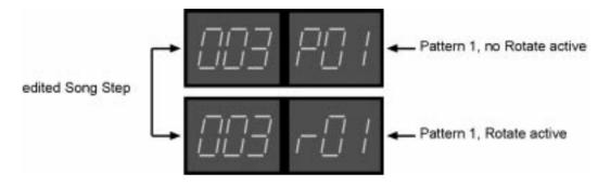
Please note: The function Song Edit - Rotate is used to select which Rotate setting is active.
